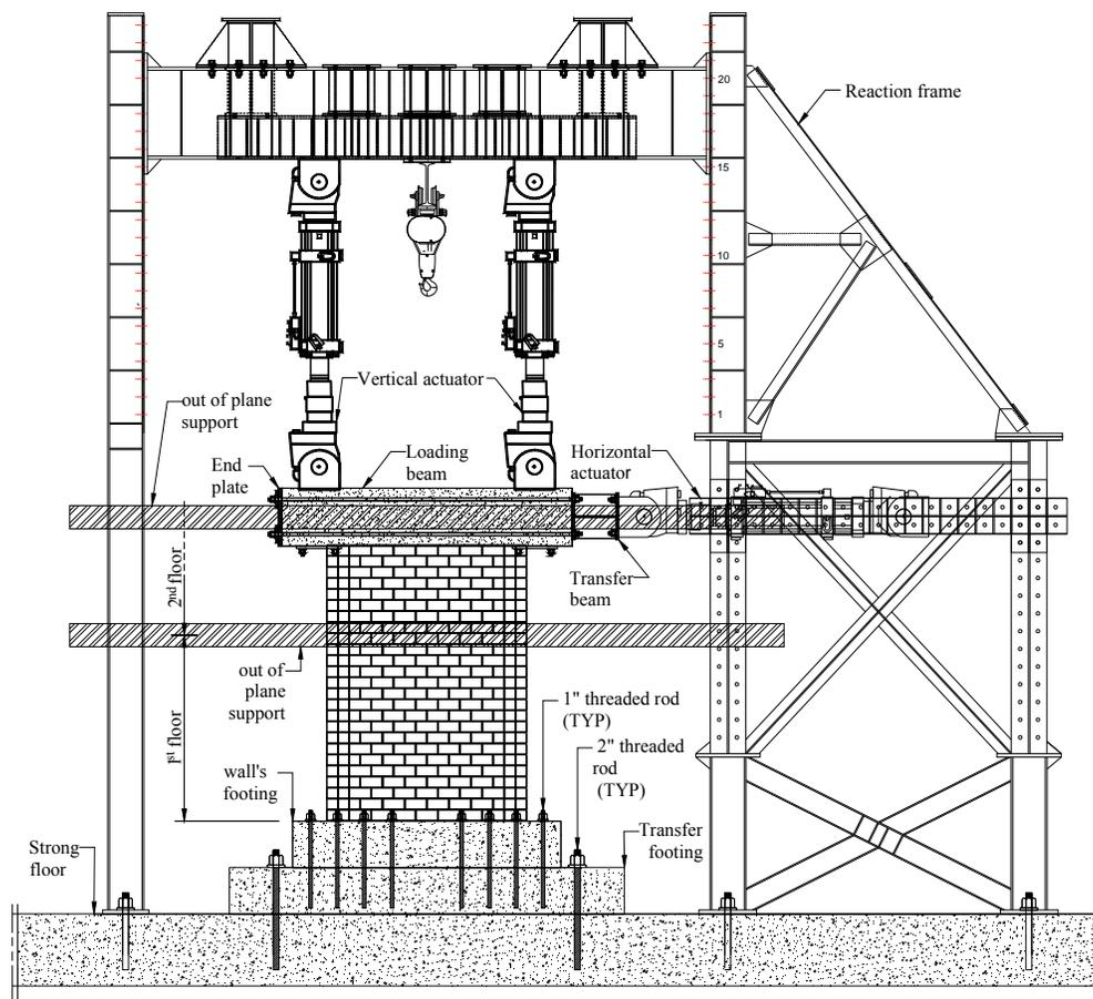
Figure 3. Test set-up
