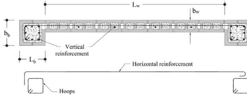
Figure 2. wall's reinforcement details
