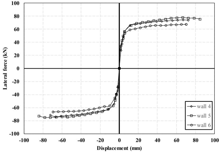
Figure 5. Effect of changing boundary element length and vertical reinforcement ratio.
