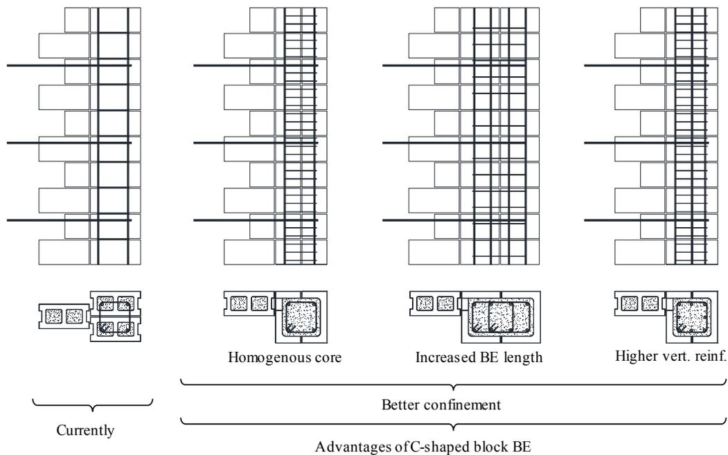
Figure 1. Advantages of C-shaped block boundary elements
