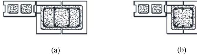
Figure 6. reinforcement arrangement in boundary elements: (a) 190 x290 boundary element, (b) 190x190 boundary element.
